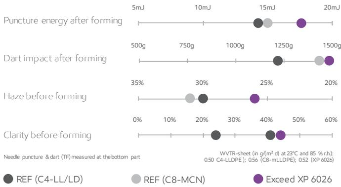
Regular blown case. Thermoforming parameters (TF): no plug/vacuum forming, temp. 100°C, 9 cm depth, DR 3.6 (deep draw).
