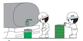
Provide the drum/container to collect the remnant .Visual checking through foot valve (for non DG only)
