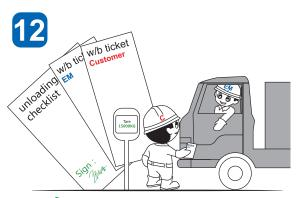
Pass one copy of weighbridge ticket to driver and keep one .Sign off the unloading checklist with the actual receiving quantity
