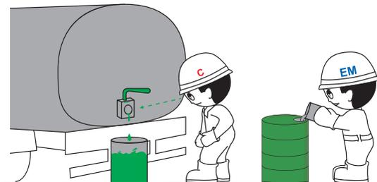
✓ Provide the drum/container to collect the remnant. Visual checking through foot valve (for non DG only)
