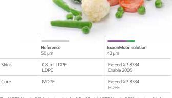
C8-mLLDPE (density 0.916 g/cm³, melt index 1.0 g/10 min); LDPE (density 0.923 g/cm³, melt index 0.3 g/10 min); HDPE (density 0.961 g/cm³, melt index 0.7 g/10 min); MDPE (density 0.931, melt index 0.2 g/10 min)
