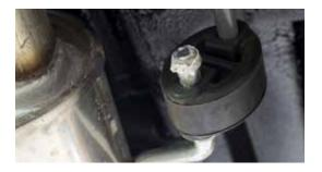
The exhaust hanger on a vehicle must withstand very intense environmental conditions while maintaining flexibility and dampening vibrations. Exxon<sup>™</sup> chlorobutyl is an excellent material to meet these requirements in order to maintain your exhaust system and prevent component failure.
