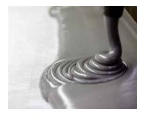
Cement formulated with Exxon™ bromobutyl grade 2222 provides a watertight seal that remains flexible across a wide range of temperatures with minimal shrinking during cure.
