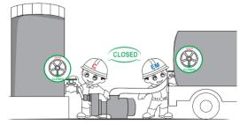
Making or breaking connections, cooperation between driver and operator is very important to avoid incidents
