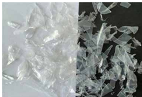
Picture 1 - Almost colorless recyclate
