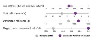
In summary, using the latest generations of performance PE from ExxonMobil and SoarnoL DC3203RC, it is possible to create >95%¹ PE-based pouches for edible oil packaging, while maintaining packaging integrity, optics, machinability and packaging line speed during VFFS operation.
