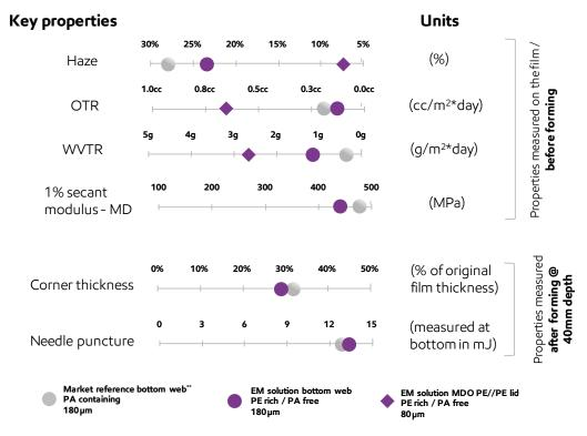
\*\* PE/Tie/coPA/EVOH/coPA/Tie/PE with thickness distribution: 45/20/20/10/20/20/45, with 22% coPA and outer PE layer based on LLDPE and sealant PE layer based on Exceed 1018.
