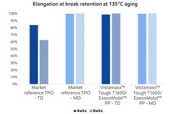
TD: Transverse Direction MD: Machine Direction
