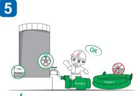
Check tank valve status; Verify tank capacity and sign name on unloading checklist
