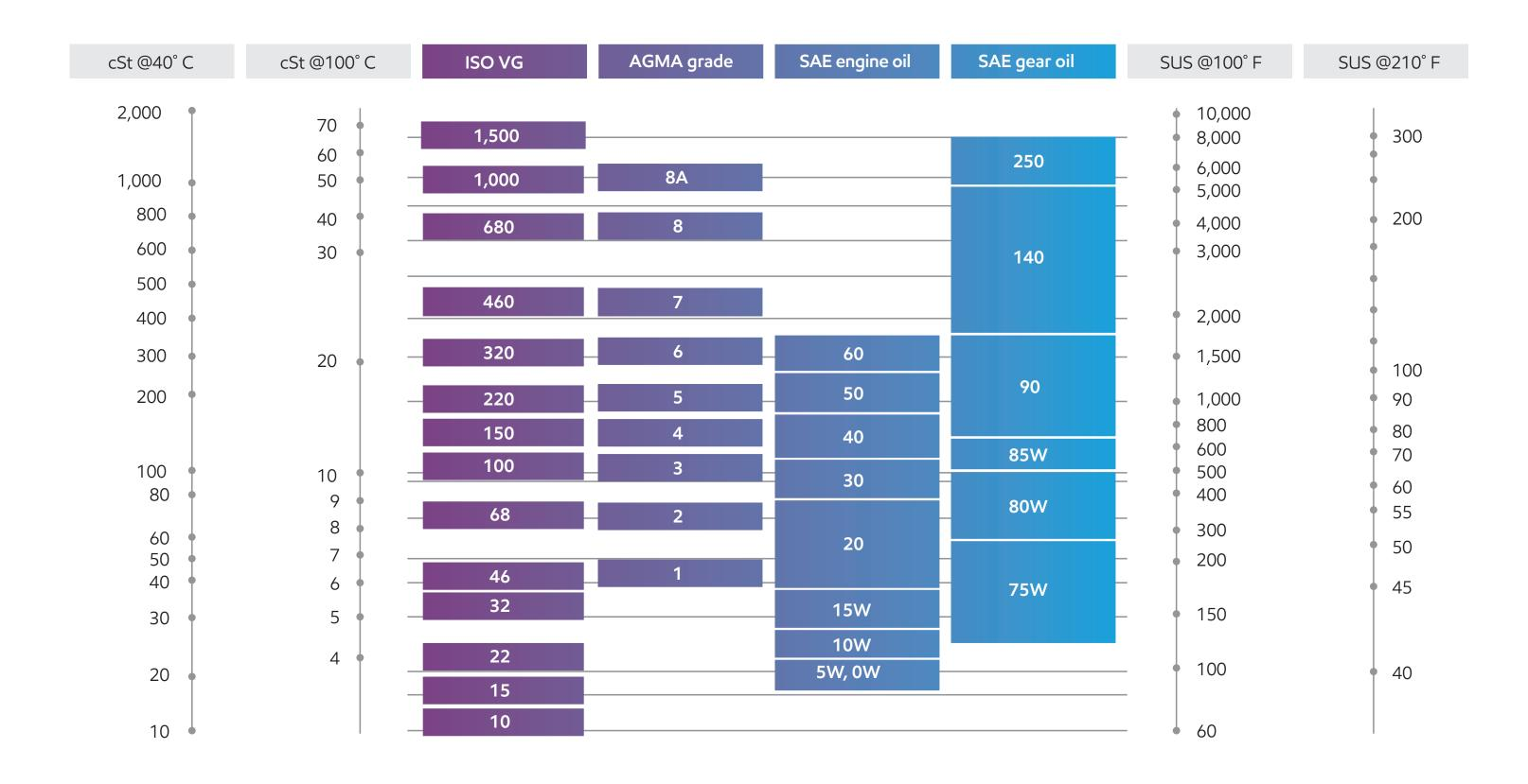
This is a rough guide for comparing equivalent viscosities under different classifications. Viscosities are related horizontally only.
