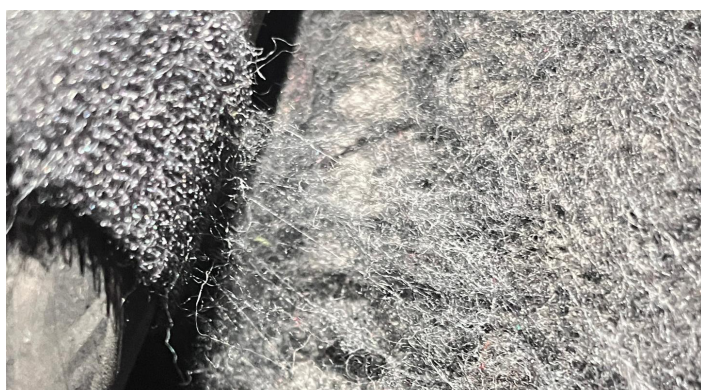
Figure 1: Floorboard Damage by using hook and loop fastener
