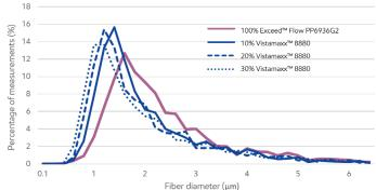
Fabrics made on single M beam Reicofil® line at 25 gsm Data traceability: BCT-201601.0177-01, BCT-201601.0177-03, BCT-201601.0177-03
