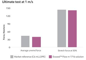
• Lower unwind force and stretch force to ease film handling by operators
