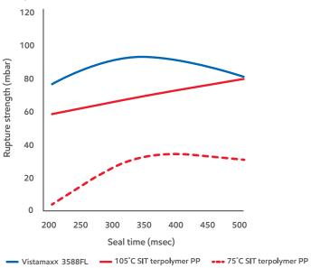
Tested at  $110^{\circ}$ C seal temperature in laminated structure:  $20\mu m$  BOPP / adlam /  $25\mu m$  BOPP sealant
