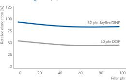
COPPCO model simulation based on UL1581 Formulation: S-PVC 100 phr, DOP or DINP 25-95, CaCO<sub>3</sub> 50 phr. Condition: Dumbbell specimen: ~1mm forced ventilation oven aging for 7 days at 100°C with air exchanged ~125 times/hr.
