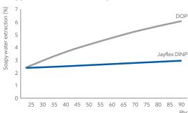
COPPCO simulation: Soapy water extraction based on ASTM D1239 Formulation: S-PVC 100 phr, DOP or DINP 25-95, CaCO, 50 phr.
