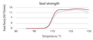
● Solution based on Exxtra™ Seal, Exceed™ Stiff+ and Exceed™ performance PE
