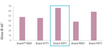
The above graph represents gloss levels of compounds when test specimens were molded using A1 surface mold polish.
