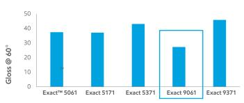
The above graph represents gloss levels of compounds when test specimens were molded using A1 surface mold polish.
