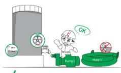
Check tank valve status; Verify tank capacity and sign name on unloading checklist
