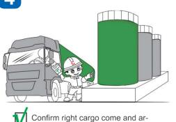
range proper tank to receive
