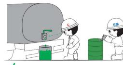
Provide the drum/container to collect the remnant .Visual checking through foot valve (for non DG only)
