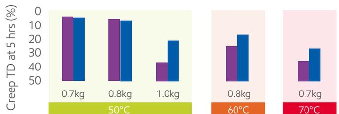
Lower creep at higher temperature and higher load up to **140°C**
